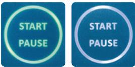
Pa stop/pause, press the START PAUSE button once. Pressing one of the two programme selection buttons also puts the device into pause mode. The green illuminated LED ring and the writing change to white and the toe flap immediately returns to
