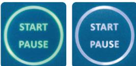
When the planned treatment time of 25 minutes is reached (i.e., the display has counted down from 25 to 0 min), the LED ring and the writing turn white.
