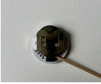
use non-conductive tool to remove
